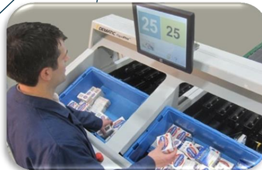
GOODS TO PERSON STATION
